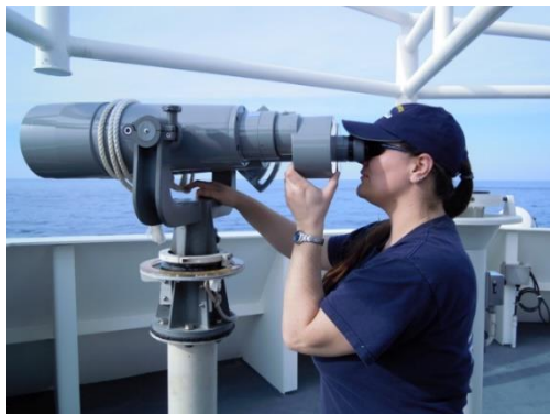
Left. Standard US Fisheries and Japanese commercial visual BIG EYES detection system for marine mammals
