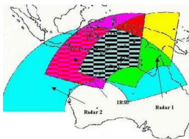
Radar 2 (blue arc) is located at Laverton IRSU (pink arc) is the Jindalee Alice Springs Facility Radar 1 (yellow arc) is located at Longreach
