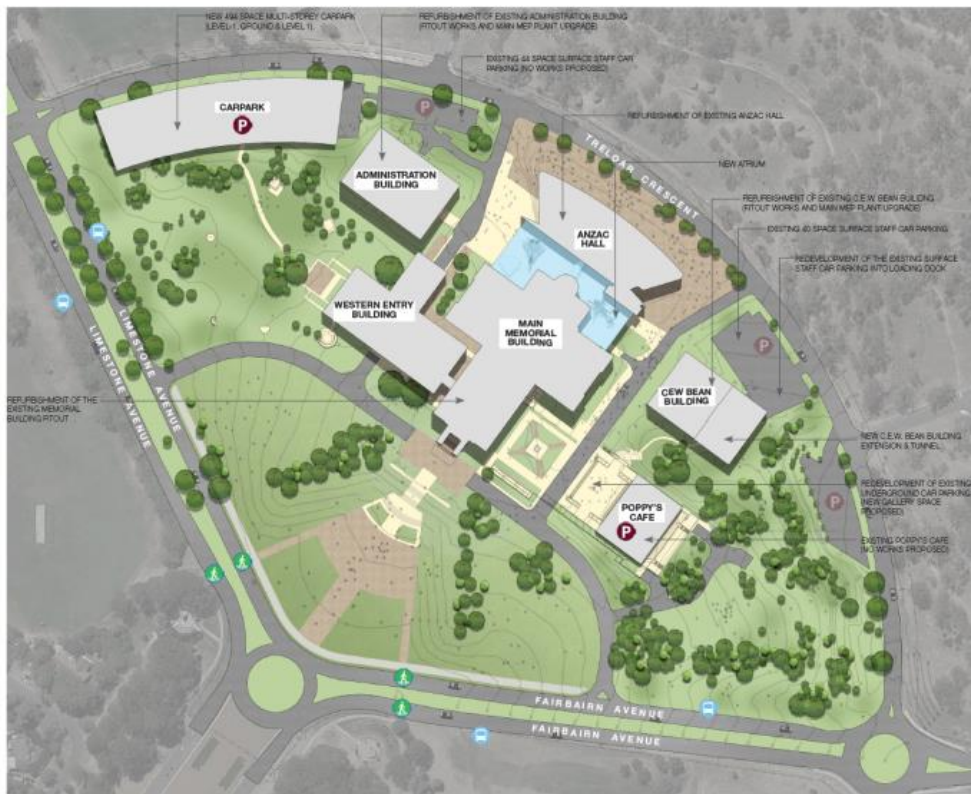
Figure 3-4 – Option 4 New entrance pavilion to the west and gallery space underground to the east
