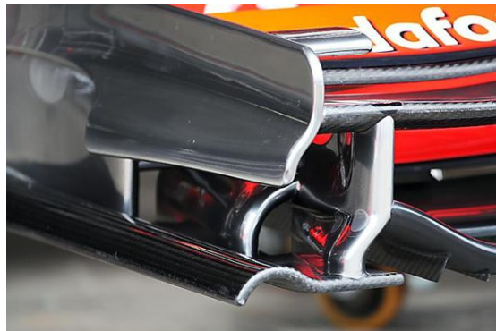
Aerodynamic detail of the front wing end plate of the 2009 McLaren F1 car
