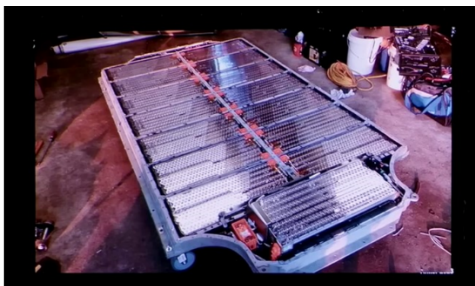
The battery floor of an EV.
