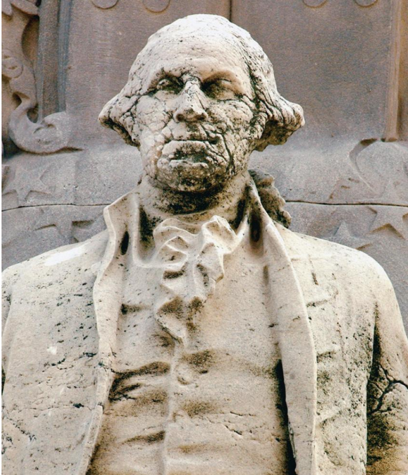
Figure 1. The impact of acid rain on the statue of the Lincoln Memorial in Washington DC.
