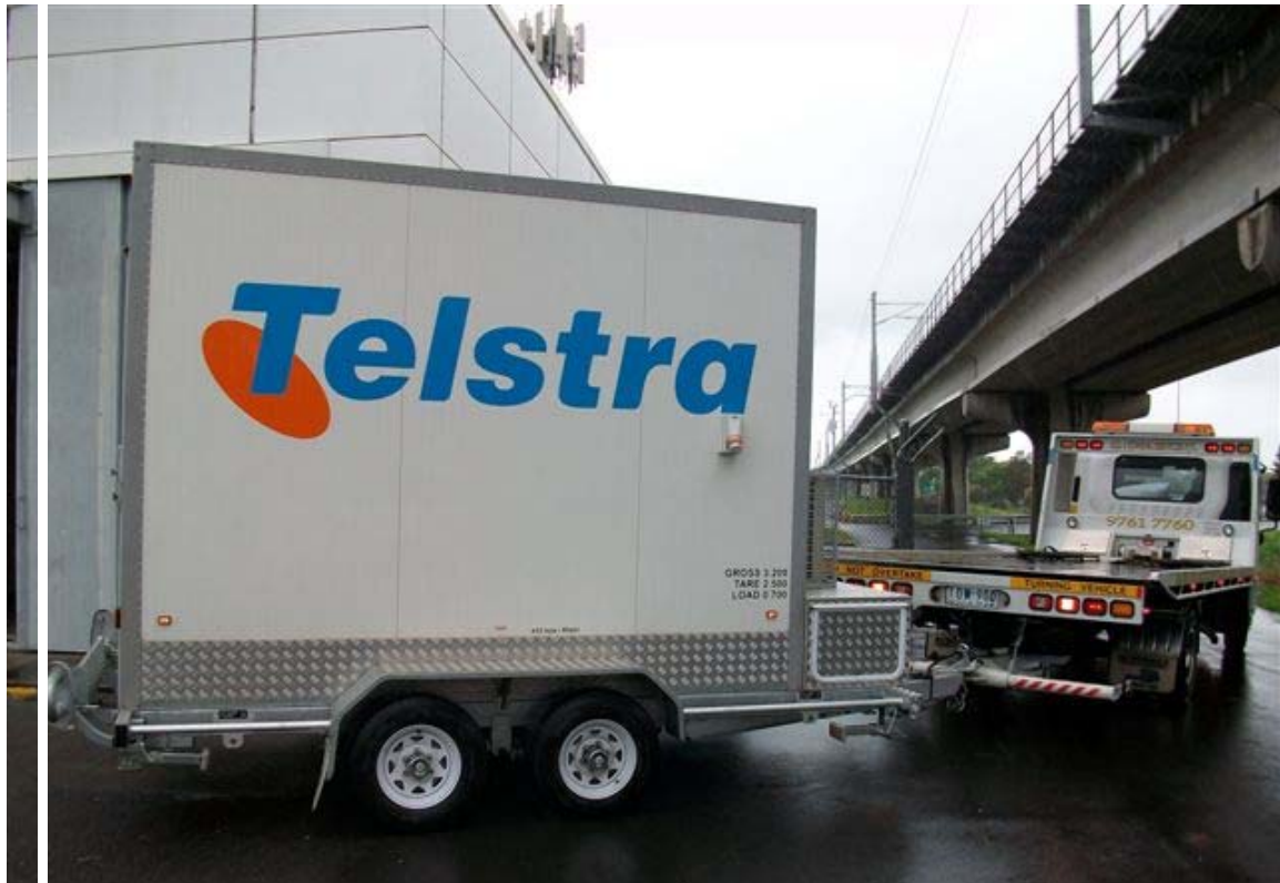
Figure 4: A Cell On Wheels (COW) on the move to a new location. These portable cell sites can be rapidly deployed in an emergency event to provide supplementary mobile coverage to ESOs and the local community.
