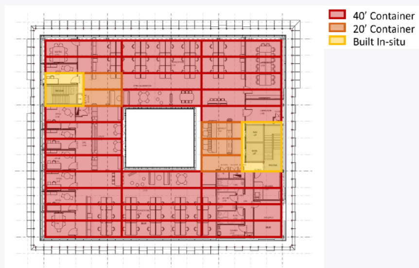
Diagram of the proposed Prefabricated Methodology
