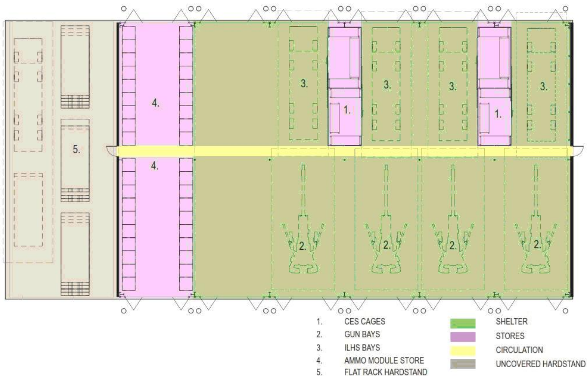
Robertson Barracks, Darwin - VEHICLE SHELTER - GROUND FLOOR PLAN SCALE: 1:200 at A4 0 4000 8000
