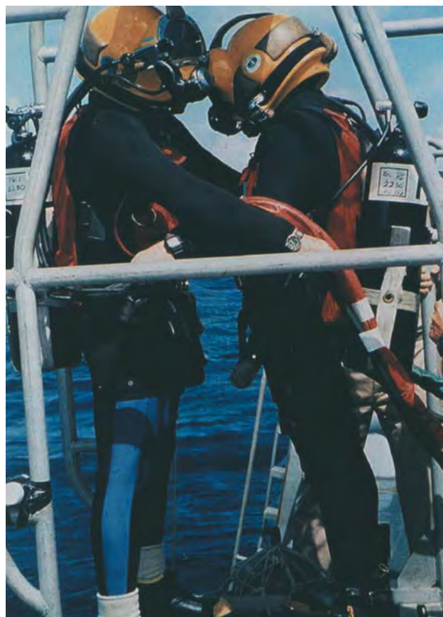
Fig. 31-1. Both divers are wearing the US Navy Mark (Mk) 21 Mod 1 Underwater Breathing Apparatus for helium-oxygen diving to 90 msw (300 fsw). Reprinted from US Department of the Navy. US Navy Diving Manual . SS521-Ag-PRO-010. Washington, DC: Naval Sea Systems Command. Rev 4 (20 Jan 1999); Change A (1 Mar 2001); p13-12. NAVSEA 0994-LP-100-3199.
