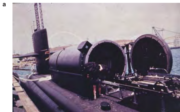
Fig. 37-12. (a) A Dry Deck Shelter (DDS) is being installed onto a host submarine. (b) US Navy SEAL ( sea, air, land ) divers launch a SEAL delivery vehicle (SDV) from the DDS. Photographs: Courtesy of US Special Operations Command, MacDill Air Force Base, Tampa, Fla.
