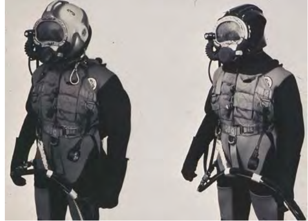
Fig. 31-9. The US Navy Mark (Mk) 21 Mod 0 helmet with hot water suit (left) and Mk 22 Mod 0 band mask with hot water suit and shroud (right) for heating breathing gases. These are the primary underwater breathing apparatuses for saturation diving. Reprinted from US Department of the Navy. US Navy Diving Manual . SS521-Ag-PRO-010. Washington, DC: Naval Sea Systems Command. Rev 4 (20 Jan 1999); Change A (1 Mar 2001): p15-6. NAVSEA 0994-LP-100-3199.
