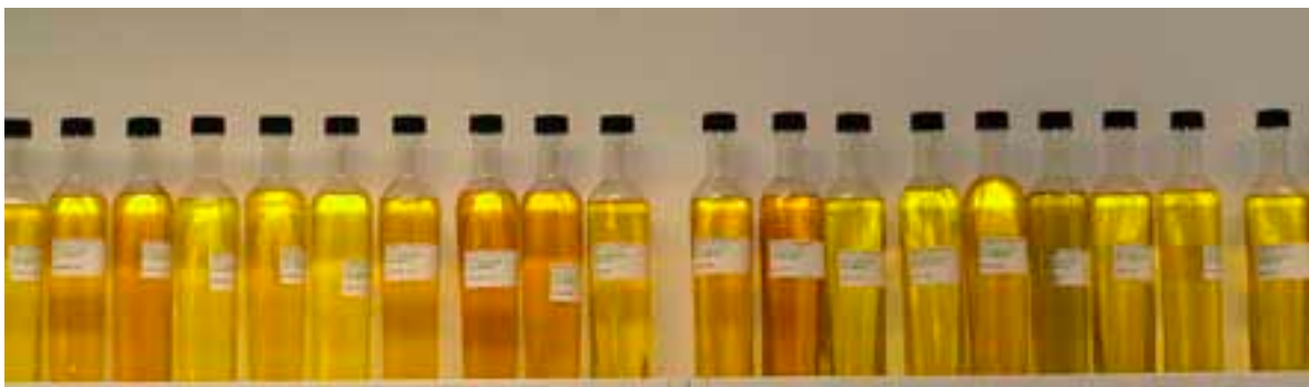
Figure 3.2 Samples stored in clear bottles and exposed to light to determine the influence of light exposure on olive oil quality
