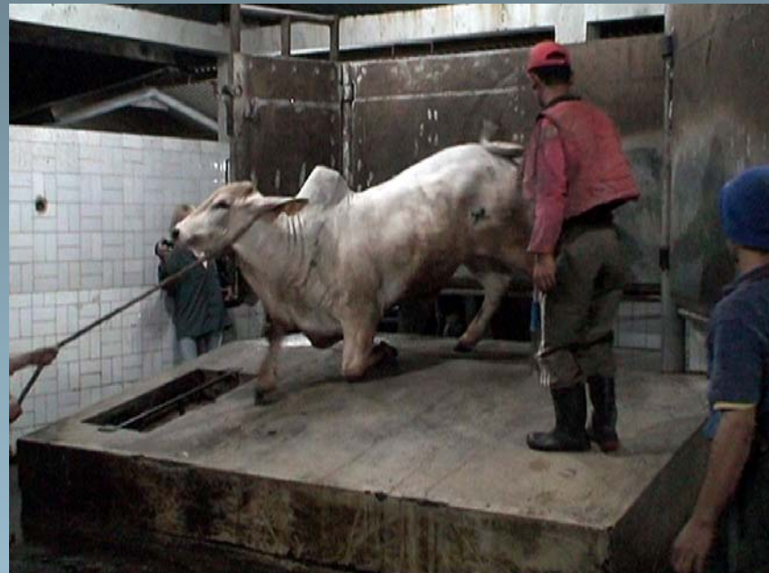
Figure 5 Tripping and pulling a steer over after opening a Mark 1 restraint box
