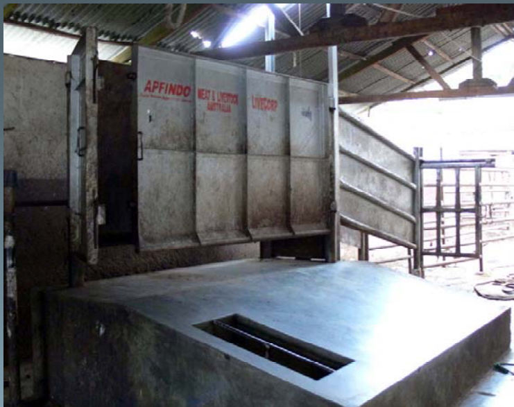
Figure 1 Mark 1 restraint box with blood drain, installed in an Indonesian slaughterhouse
