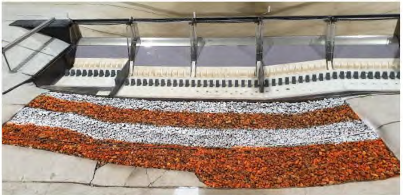
Figure 16 Removable bed scour test, prior to run (note spray-painted gravels)
