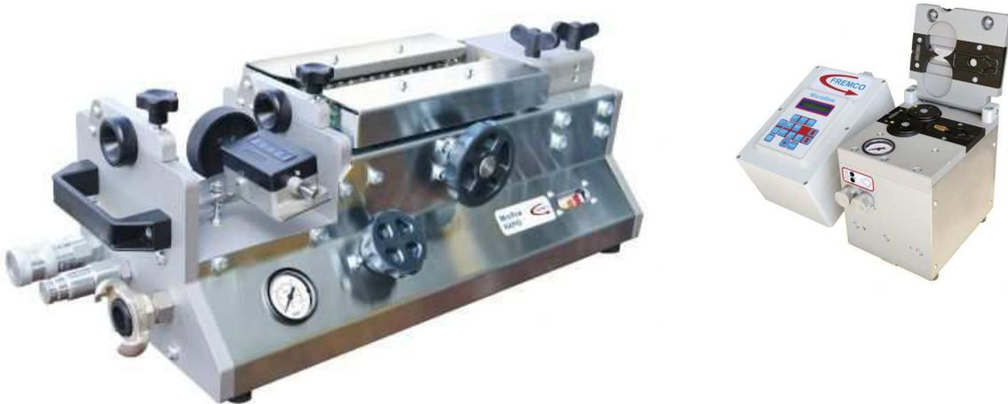
The above two cable “Blowing” machines / tools<sup>11</sup> are examples of this relatively new technique. The much larger unit (above left) is for main/thick SMOF cables through large conduits and the one on the right is for FTTH in much smaller conduits, ie into houses, home units, factories from the street. The equipment shown here may not be optimised for Australian cable and conduit dimensions.
