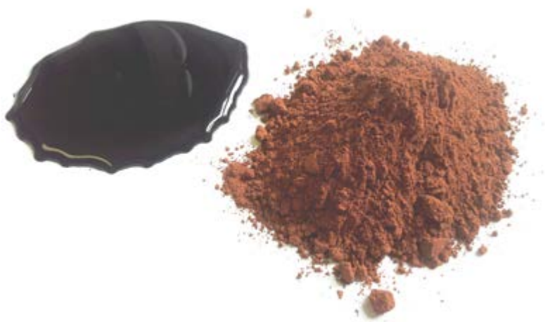
Figure 4.12: BanahCEM has two ingredients: calcined clay and a proprietary activator.
