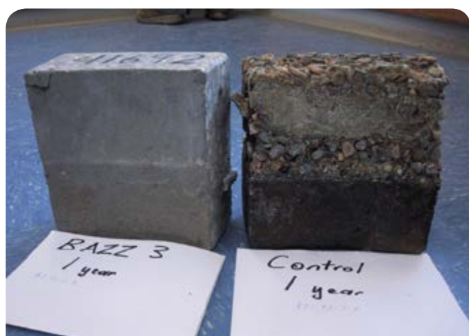
After 1 year: Left - Rocla geopolymer, Right - Portland cement concrete
