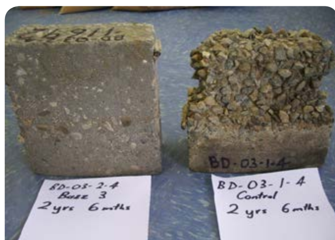
After 2 years 6 months: Left - Rocla geopolymer, Right - Portland cement concrete
