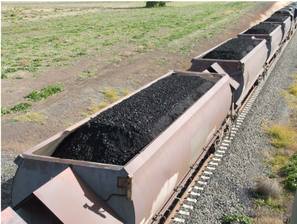
Figure 10 Photograph showing a 'garden bed' shape load profile (Photograph taken by Jim Harrison at Boggabri Coal on 13 July 2007) (extracted from Connell Hatch, 2008)
