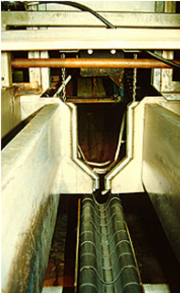
Cow's eye view of the head holding device for ritual slaughter on the center track double rail restrainer.
