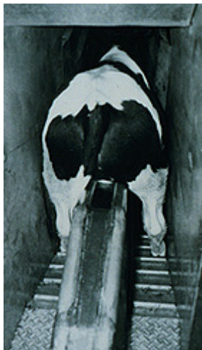
Veal calf entering the center track restrainer. For all species, it's very important to have a non-slip ramp with cleats. For adult cattle, a belly rail must be added (see diagram of cross section through the restrainer entrance).
