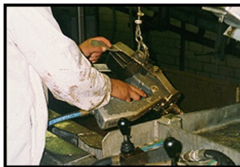
Figure 2. Pneumatic captive bolt stunner equipped with an ergonomic handle. When this stunner is used in a conveyor restrainer it should be hung at an angle.
