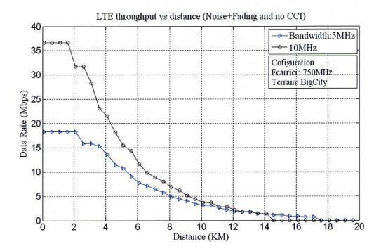
Note on above image: This simulation assumed a 10watt transmitter equipped with a directional antenna. Noise and fading are included but it is assumed there is no adjacent cell.
