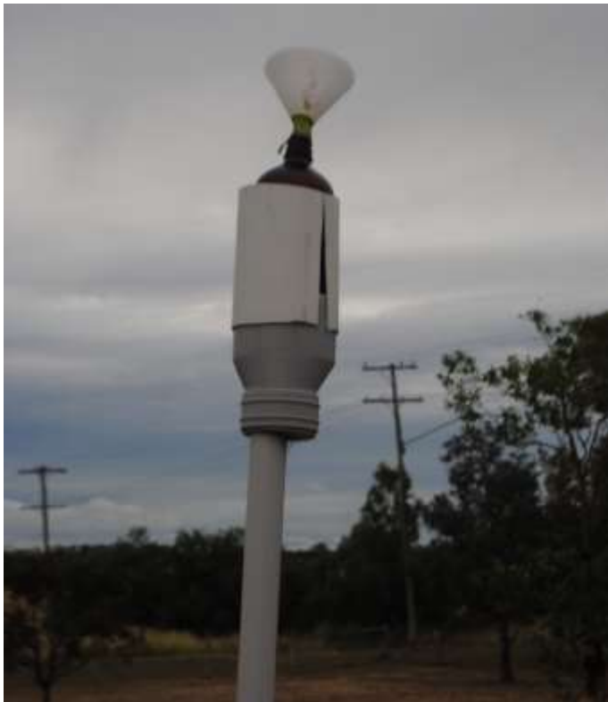
Fig 1 Dust funnel Acland. These have been known to contain anything from frogs, insects, dried grass or old rags
