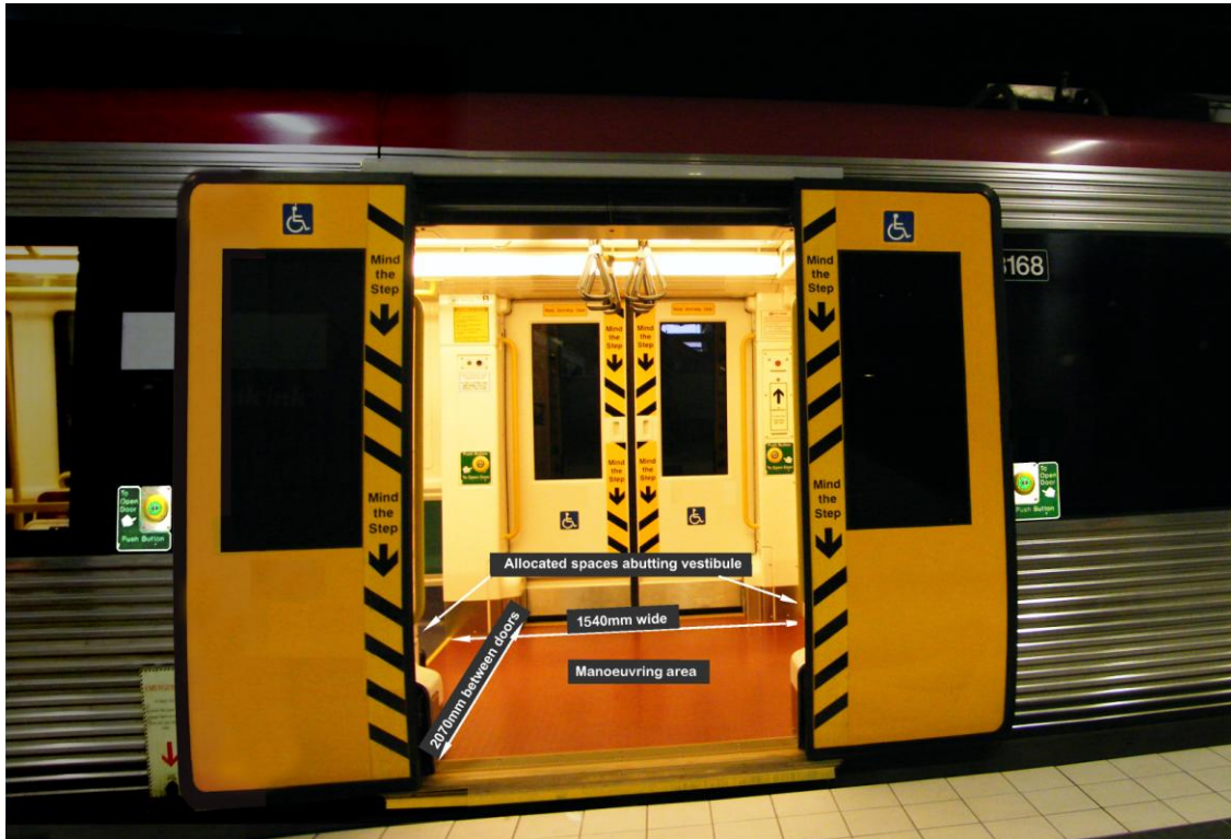
Figure 7.1.3.a. Example of circulation space dimensions in a new carriage (dimensions in millimetres). Note: Sign text may be sentence or title case.
