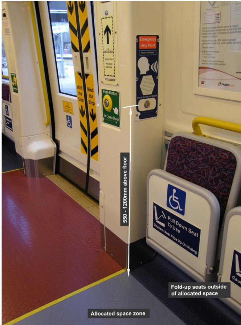
Figure 7.2.1.b. Examples of allocated space assistance control specification (dimensions in millimetres). Note: Sign text may be sentence or title case.
