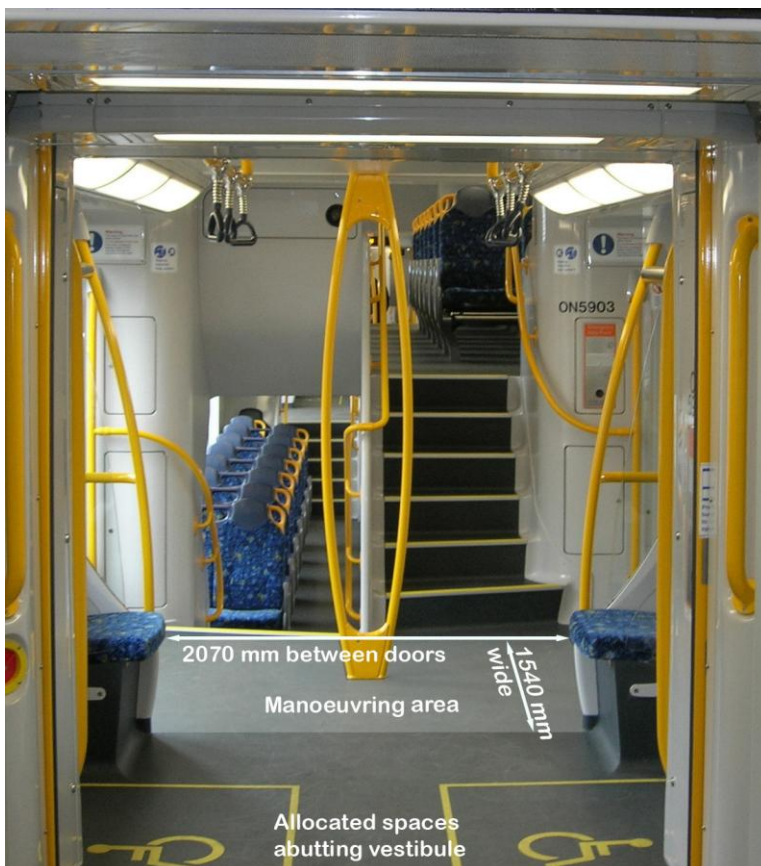
Figure 7.1.3.b. Example of circulation space dimensions in a new carriage (dimensions in millimetres).
