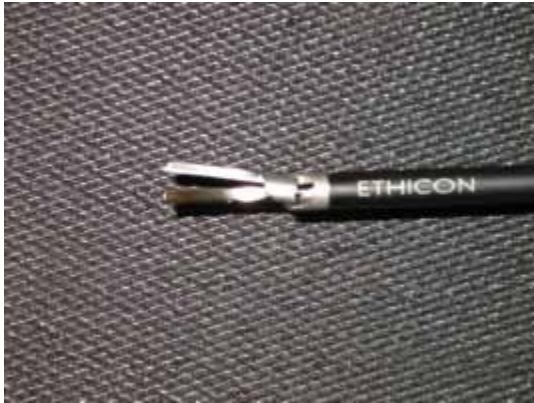
Figure 4: Automatic opening of the shears is incomplete
