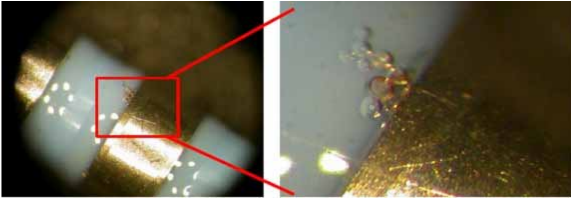
Figure 6: Air bubbles and contamination in the adhesive used to secure the electrode
