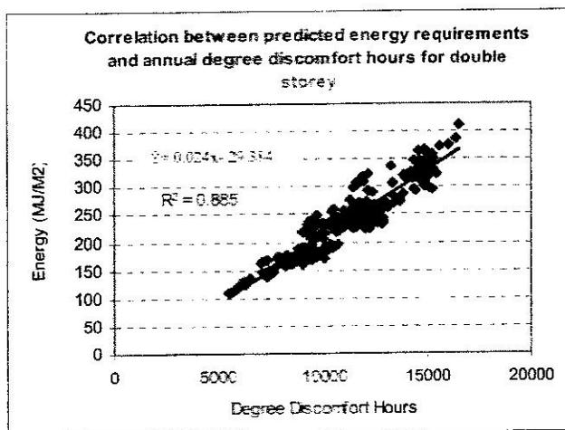
Figure 3: Correlation between indicators of thermal performance simulated double storey houses in different operation modes
