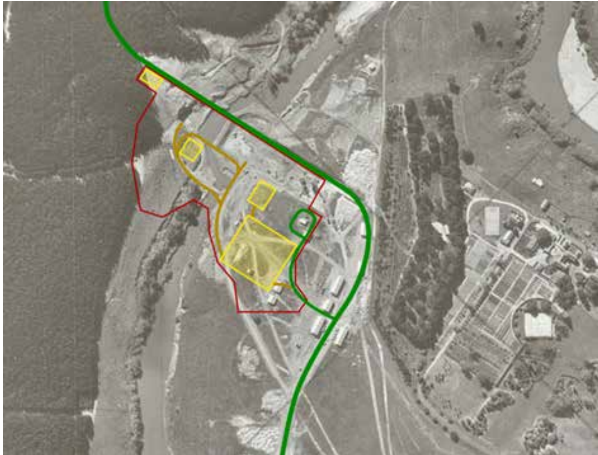
Figure 11. Existing proposed impacts over 1961 aerial image of impacts (red = potential impact areas, green = existing roads, yellow = proposed laydown areas, brown = temporary construction roads).
