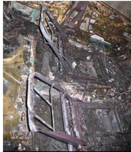
Passenger compartment (post fire)
