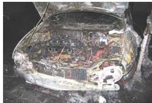
Engine compartment (post fire)
