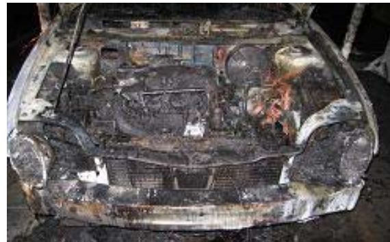
Engine compartment (post fire)
