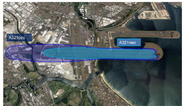
A321ceo compared with A321neo Noise footprint overlay at Sydney Airport
