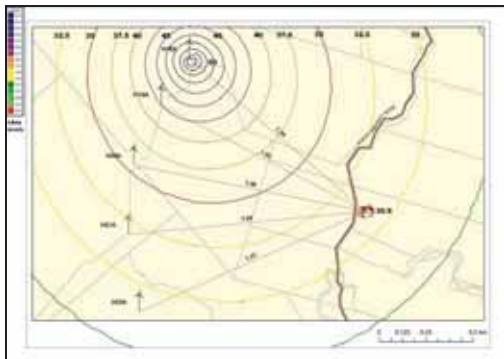
Figure 4: one turbine operating, sound level contours and predicted sound level at residence
