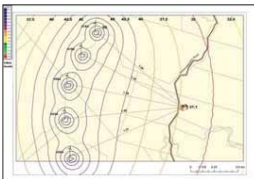
Figure 5: five turbines operating, sound level contours and predicted sound level at residence
