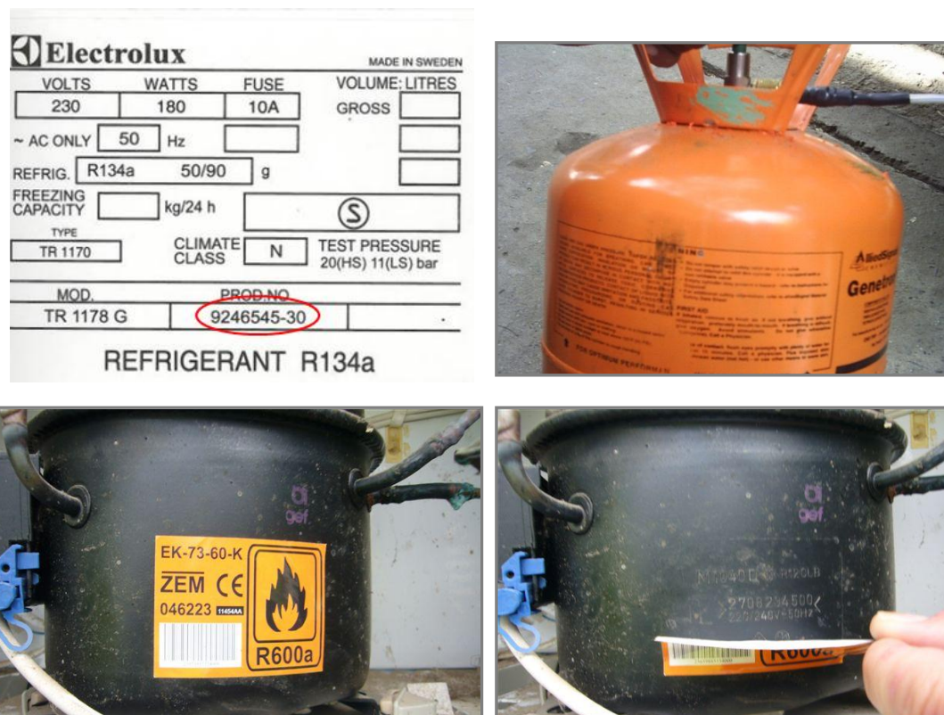
Figure 2. Concealment methods associated with pollution crime, including the use of fraudulent documents, false labels and paint.
