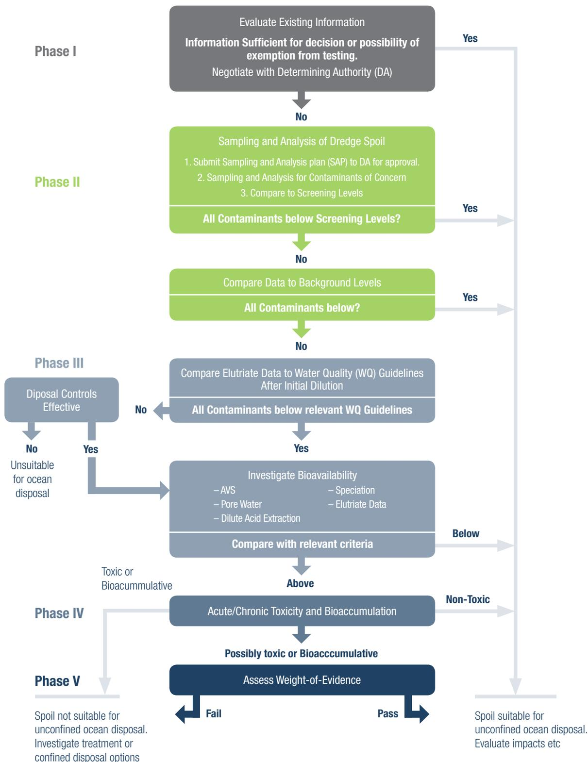
Figure 4.3: Assessment of dredged sediment and materials.
