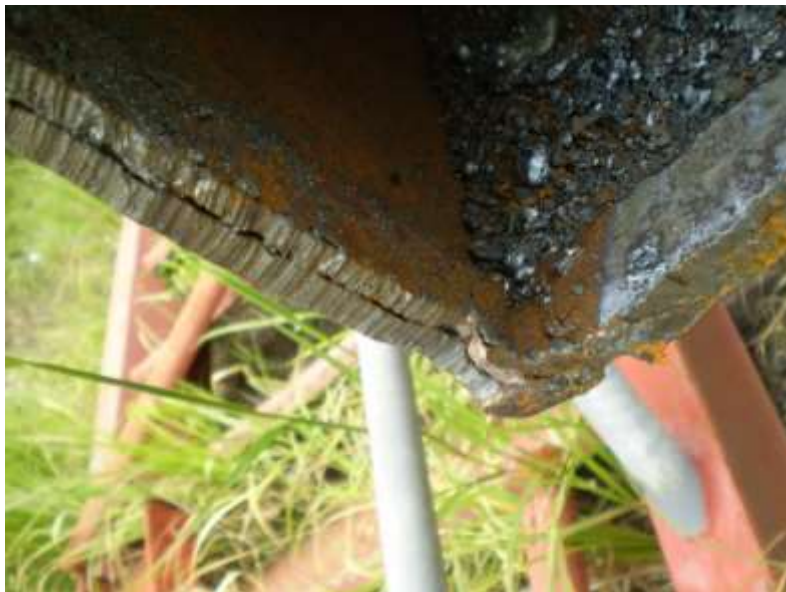
Photo 20 – 23 Under cut on weld profiles
