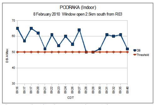
5. Indoor readings are made within a living space with one window open. Here too noise levels for almost all overflights exceed 50dB.
