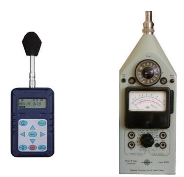
7. *Right* The **CEL-460** that was used to make the overflight noise measurements and at *left* a **Bruel Kjoer 2209** noise meter used to calibrate the CEL-460. They were found to be commensurate within a decibel in the A-band used for the overflight noise readings. The meters were loaned courtesy of the *Civil Engineering Laboratories, University of South Australia.*
