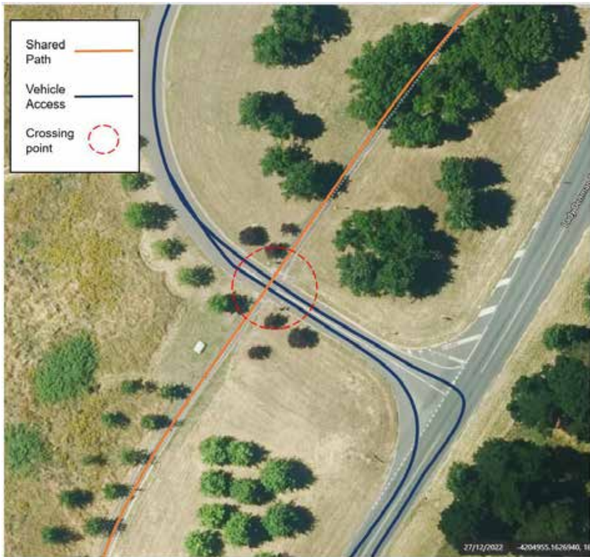
Figure 5.13 Shared path crossing with vehicle access to site. Sourced from MetroMap, modified by GHD.
