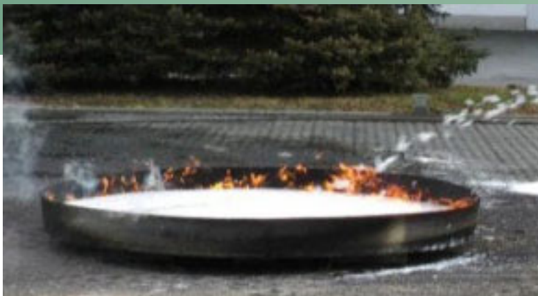
ICAO Level B fire test showing F3 edge flickers after 60seconds foam application
