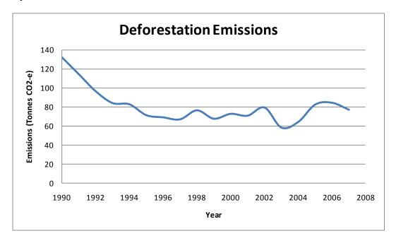
National emissions from Deforestation declined from 132 million tonnes (Mt) carbon dioxide equivalent (CO<sub>2</sub>-e) in 1990 to 77 Mt CO<sub>2</sub>-e in 2007. Much of the reduction in emissions from Deforestation since 1990 occurred before consideration of greenhouse gas emissions targets.
