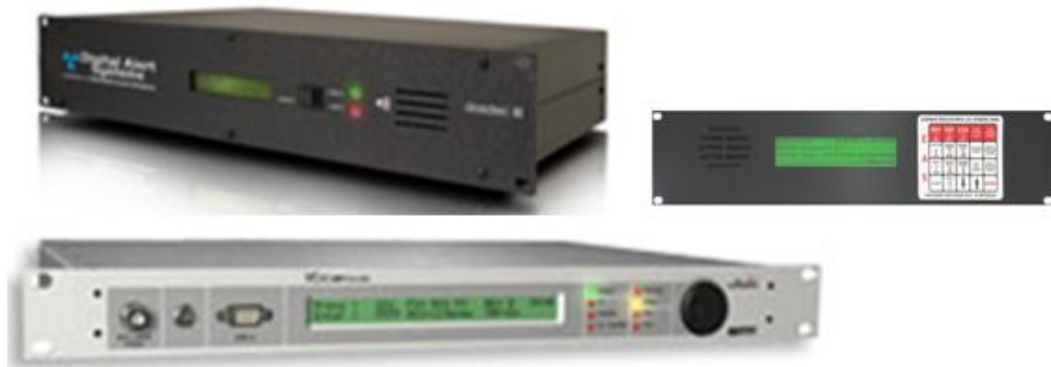
Fig 1. Sample of rack mounted RDS Encoders/Decoders
