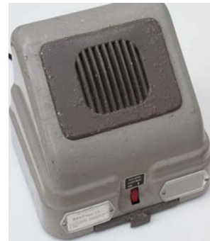
Remote battery powered receiver unit
