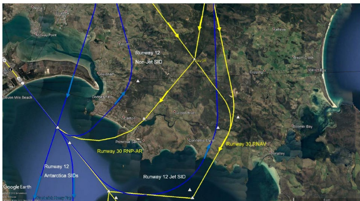
Figure 3 - Final Design (March 2019) - Zoomed in image showing Runway 12 departures and Runway 30 arrivals in the South East region; arrivals (yellow); departures (blue); waypoints (white triangles), from Airservices' Hobart-Airspace-Design-Review-Final-Report-March-2019, Figure 4, page 23.
