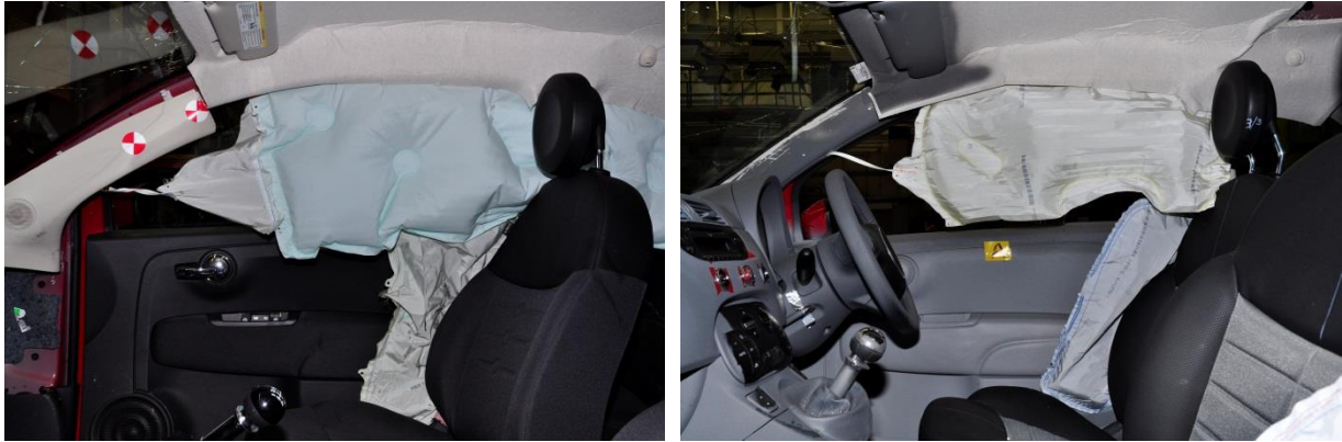
Figure 11 North American market vehicle (left) and Australian market vehicle (right) head curtain and thorax side airbags, post deployment (Model A)
