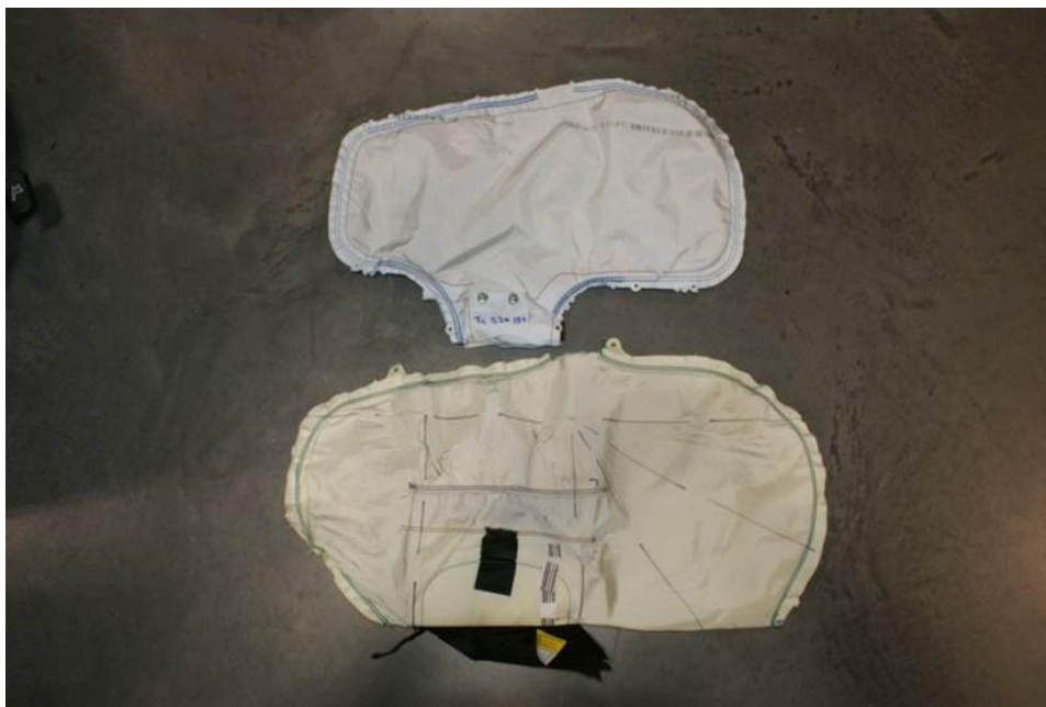
Figure 14 North American market vehicle (bottom) and Australian market vehicle (top) thorax side airbags (Model A)
