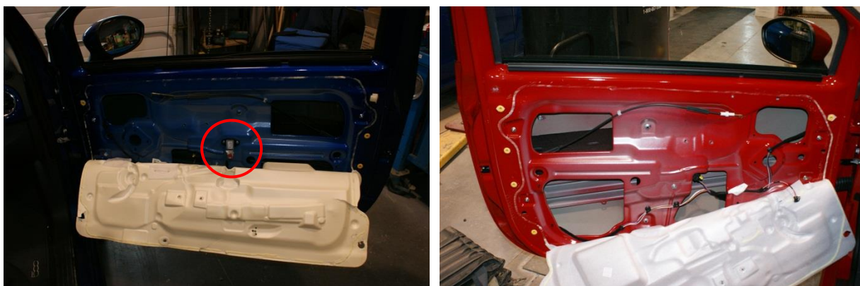
Figure 12 North American market vehicle (left) and Australian market vehicle (right) front-row door designs (note: pressure sensor (in red circle) fitted to the North American vehicle) (Model A)
