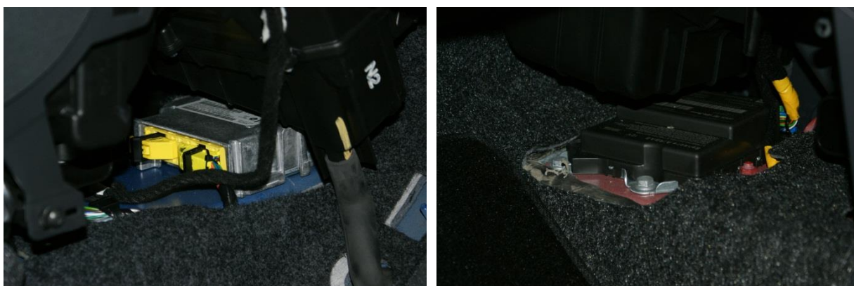
Figure 13 North American market vehicle (left) and Australian market vehicle (right) airbag control modules (Model A)
