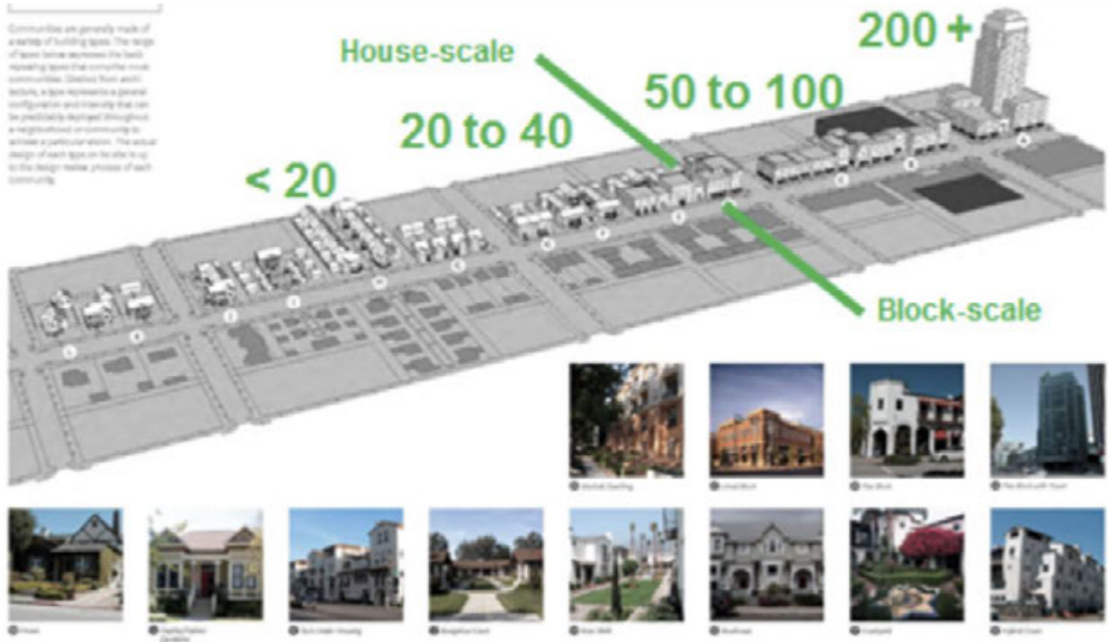
Figure 56: Form Based Code – Example of an approach to building types in relation to intensity of location (Stef Polyzoides)
