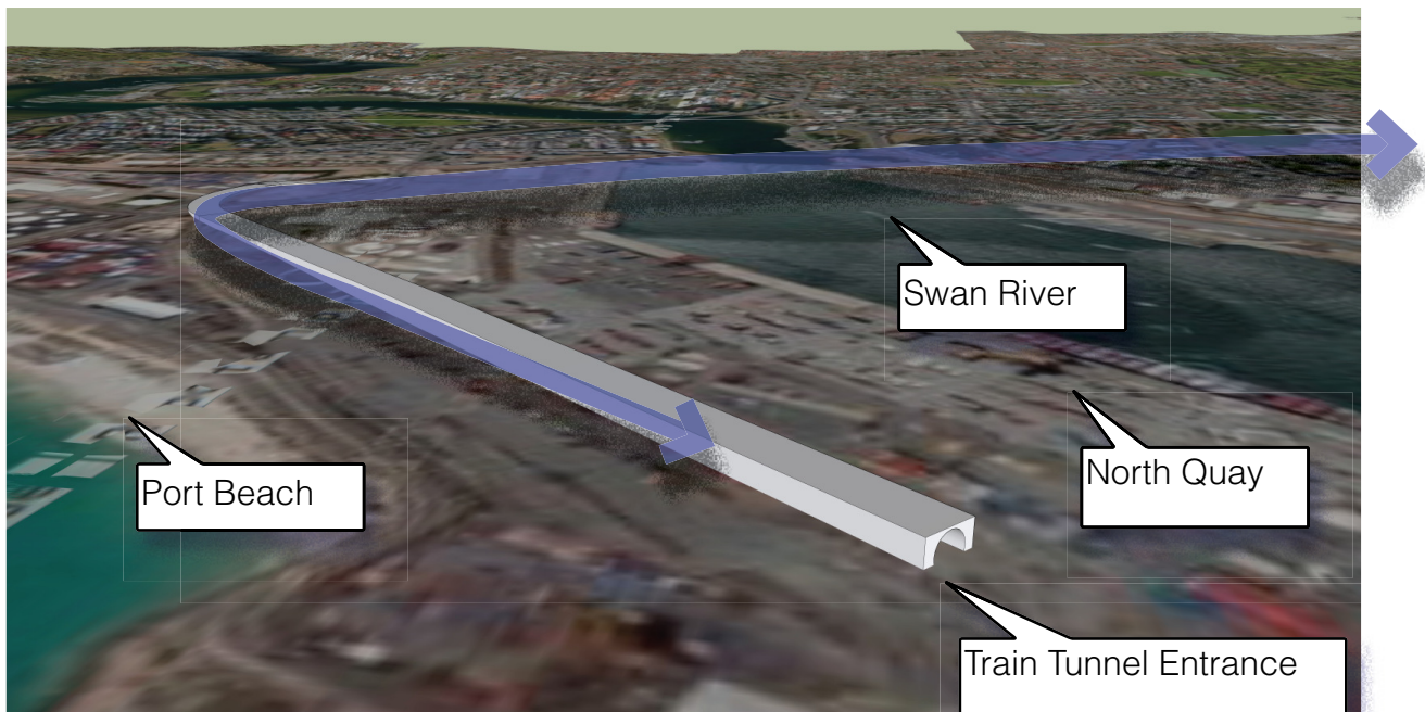
Figure 21. Rail Tunnel entrance at Port of Fremantle. Running at 1-2% grade it arrives under the river and then under Cantonment and Clontarf Hill to emerge on current rail freight corridor
