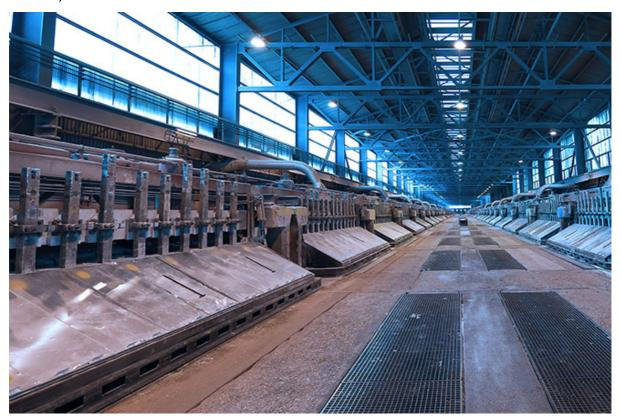
Trimet converted 120 electrolysis furnaces in its Essen aluminium smelter to trial operation as a virtual battery.
