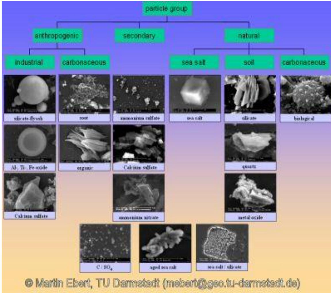
Environmental Scanning Electron Microscopy (ESEM)
