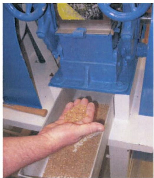
Allis Chalmers roll stands in the CGC lab have been in use for at least 80 years.
