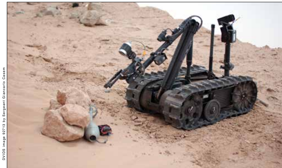
A Talon robot goes in for a closer look at a suspected improvised explosive device.
