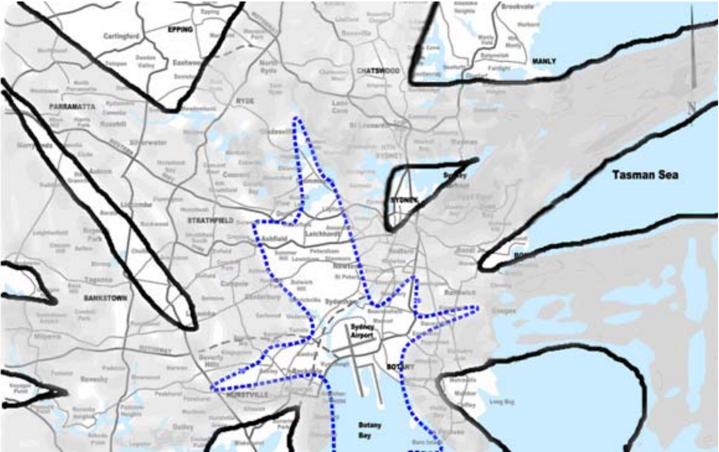
Figure 5-4 Comparison of 65 dBA Single Event Noise Contour (black) and ANEF 20 Contour (blue) for Sydney Airport
