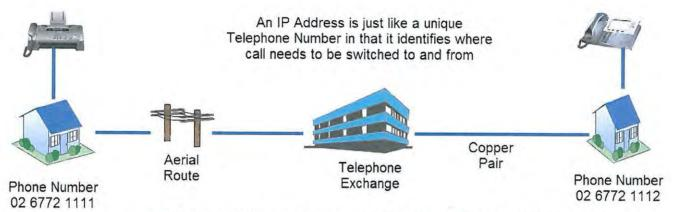
In a Telephone Network you can run out of phone numbers and copper lines so you install PABX's and Pair Gain Systems
