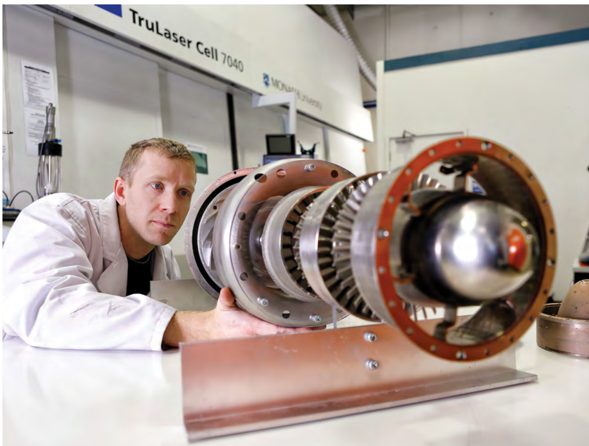
Image courtesy of Amaero. 3D printed jet engine.
