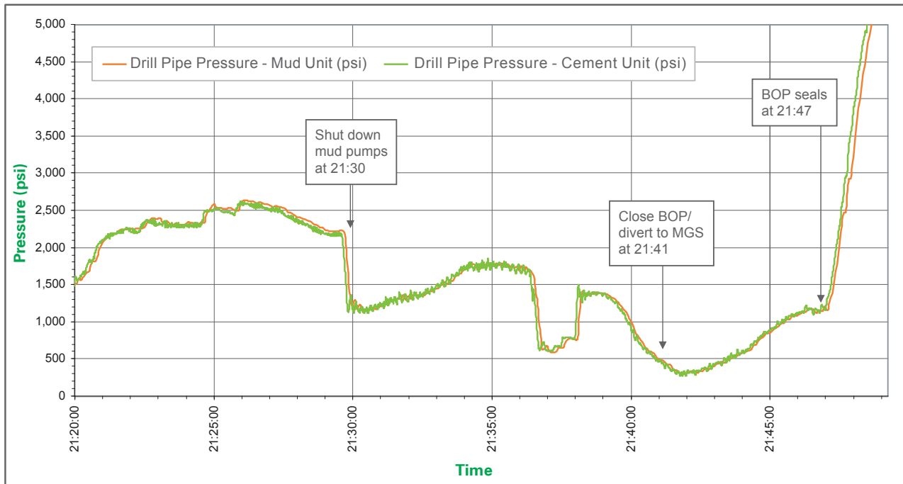
Figure 12. Drill Pipe Pressure Measured at Cement Pump PI and Mud Pump PI.
