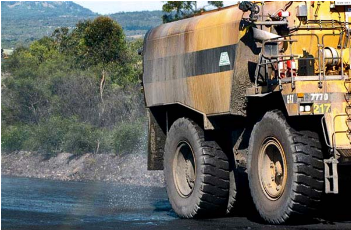
Dust suppression on a haul road (Photo: Lex Stewart/EPA)
