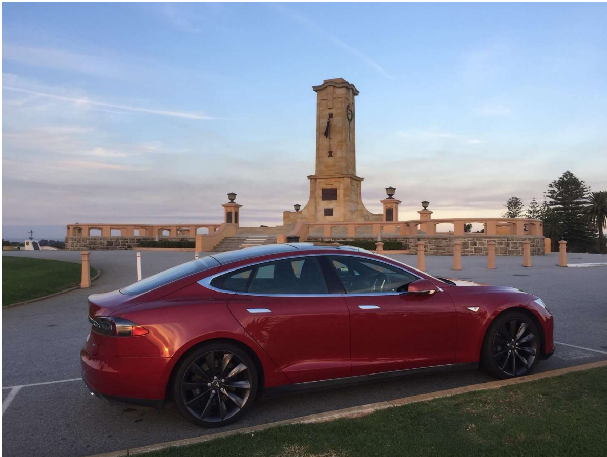
Figure 6 - 2015 Tesla Model S 85kWh. 386kW/518bhp. 400km range. Frequent software updates bring new features.
