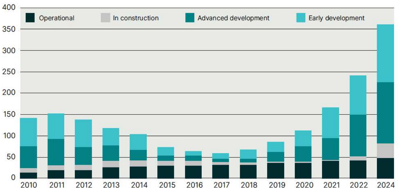
Figure 3: Pipeline of commercial facilities Since 2010 by capture capacity 5 Mtpa CO 2
