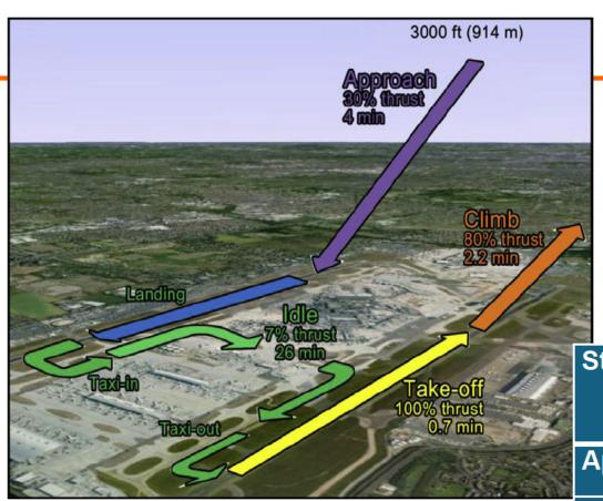
A LTO cycle refers to all the operations the aircraft carry out below 3000 ft above field elevation (914 m) which roughly corresponds to the atmospheric mixing height, i.e. the lower part of the troposphere within which pollutants emitted at ground-level mix rapidly.
